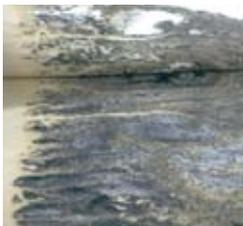
**Organics and biofouling:** Feed water with high organic matter content is the cause of these deposits. The presence of such compounds also facilitates biofilm formation on the surface of the membranes, and is the most commonly occurring type of fouling.
