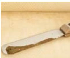
**Colloidal Fouling:** Colloids present in the feed water should normally be removed by the pre-treatment system; failure or poor design of pre-treatment systems may lead to colloidal membrane fouling.
