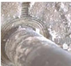
**Inorganic scale deposits:** The most common types of scale found in membranes are calcium carbonate and calcium sulphate with barium and strontium sulphate occurring less frequently. Scale can often be attributed to incorrect antiscalant selection or poor
